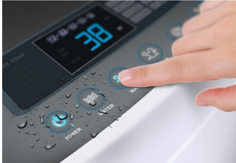
Figure 2-14. Liquid-Tolerant CapSense-Based Touch User Interface in a Washing Machine
