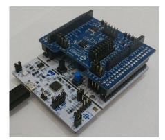
Figure 11. CY15FRAMKIT-002 mounted on ST MCU Evaluation Board
