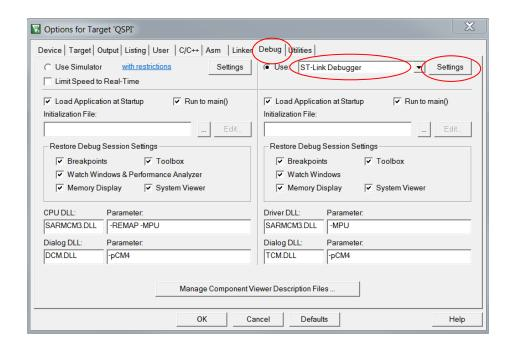
9. Click "Debugger – Settings" to select the appropriate Flash Programming Algorithm for this device
