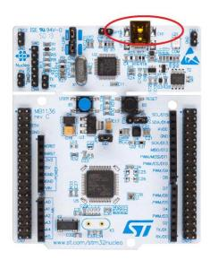
Figure 13: Connector CN1 for Nucleo 64 board
