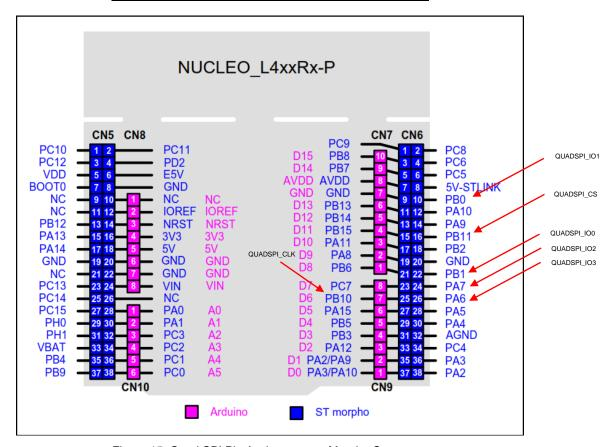
Figure 15: Quad SPI Pin Assignment on Morpho Connector
