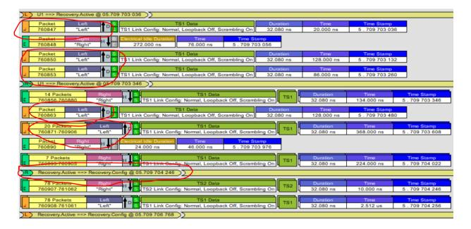
3. Later, device enters to Recovery. Configuration as shown below
