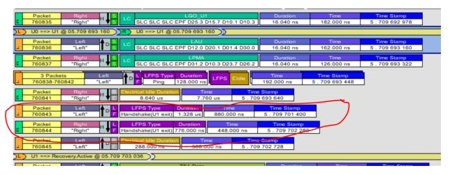
The port in SuperSpeed operation shall transition to Recovery. Configuration after eight consecutive and identical TS1 or TS2 ordered sets are received.
