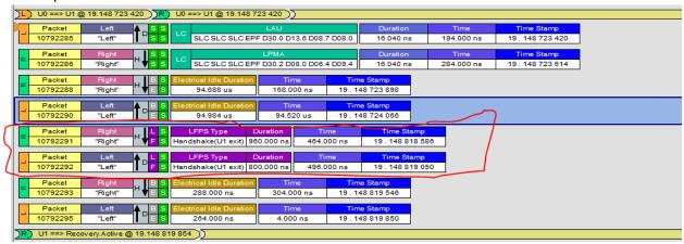
2. Device has seen 8 consecutive and identical TS1 from the host and entered into Recovery.Config. Then Device started sending TS2s.
