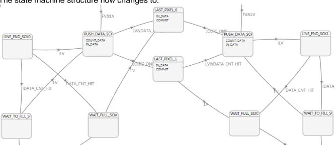
Here, the PUSH DATA SCK x states read data until the counter hits after which the LAST PIXEL x state reads the last word and commits the buffer.
