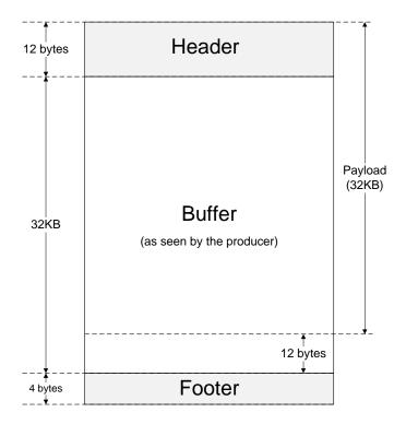
In this strategy, the GPIF state machine must be modified to fill 32K-12 bytes of data. Since this will not cause the buffer to be filled, the committing process will not happen automatically and so the COMMIT action must be used to force a wrapup.
