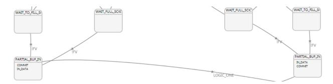
Since a partial buffer is always produced, both the WAIT states will transition to a PARTIAL\_BUF\_IN\_SCK\_x state which commits the last buffer whilst reading in 1 word of data. This is to prevent a ZLB.
