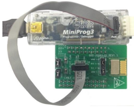
Figure 136. CYBLE-014008-EVAL Using CY8CKIT-002 MiniProg3 and 10-Pin Ribbon Cable
