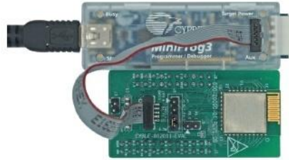
Figure 124. CYBLE-012011-EVAL Using CY8CKIT-002 MiniProg3 and 10-Pin Ribbon Cable
