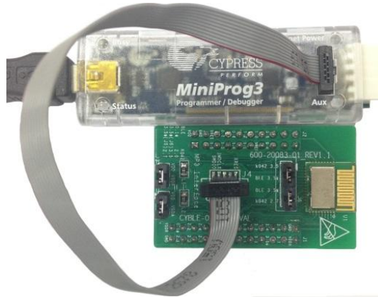
Figure 142. CYBLE-224110-EVAL Using CY8CKIT-002 MiniProg3 and 10-Pin Ribbon Cable
