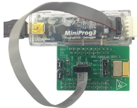
Figure 139. CYBLE-214009-EVAL Using CY8CKIT-002 MiniProg3 and 10-Pin Ribbon Cable
