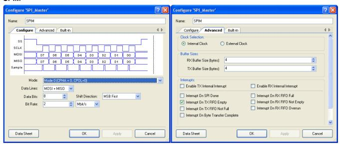
The SPIM is configured to transfer at the rate of 2 Mbps with mode 0.
