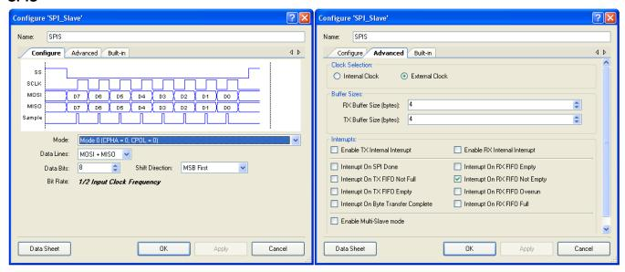
The SPI slave is configured for the same Mode 0, Data bits, and Shift Direction, as the SPI master. Interrupt on RX FIFO Not Empty is enabled so that the interrupt line goes high when a byte is received from the SPI master. This acts as the trigger for DMA Rx to move data from the SPI slave Rx FIFO to the slaveRxData buffer.
