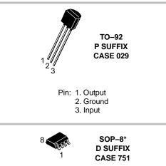
\*SOP-8 is an internally modified SO-8 package. Pins 2, 3, 6, and 7 are electrically common to the die attach flag. This internal lead frame modification decreases package thermal resistance and increases power dissipation capability when appropriately mounted on a printed circuit board. SOP-8 conforms to all external dimensions of the standard SO-8 package.
