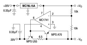
Figure 10.  $\pm$  15 V Tracking Voltage Regulator
