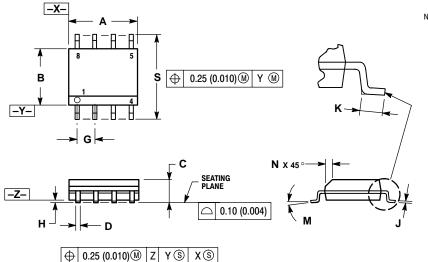
NOTES: 1. DIMENSIONING AND TOLERANCING PER ANSI Y14.5M, 1982. 2. CONTROLLING DIMENSION: MILLIMETER.
