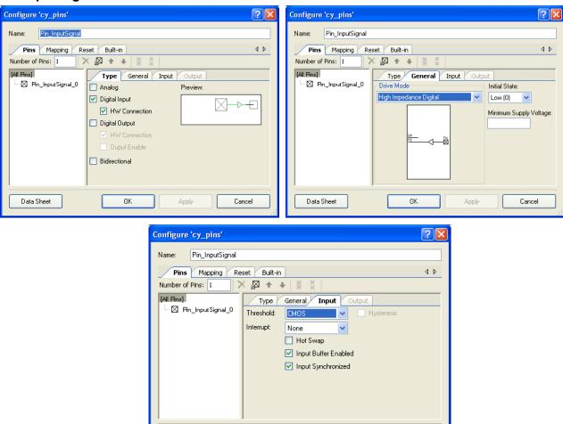
The **Pins** tab shows that the pin is a digital input. Because the pin is controlled by hardware, HW Connection is enabled. If HW Connection is disabled, the pin can be read only by firmware. The **General** tab shows that the pin is configured for High Impedance Digital drive mode.
