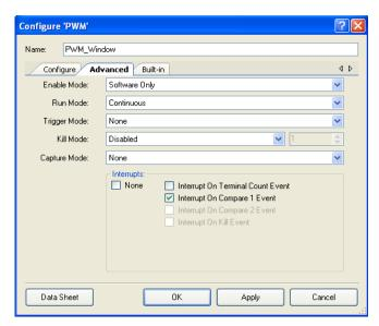
The PWM is designed using UDB. The Fixed function PWM also can also be used. The PWM output is used to generate the time window required for the count. This PWM output acts as the input to the counter capture signal. The PWM period is configured for 9999 which results in (9999 + 1) \* 100 kHz = 100.00 ms.
