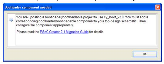
2. For Bootloadable projects, add a Bootloadable component to the design. Edit the component parameters to match your old bootloading settings.
