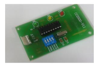
CC2500 RF Modem is a transceiver module which provides easy to use RF communication at 2.4 Ghz. It can be used to transmit and receive data at multiple baud rates from any standard CMOS/TTL source. This module is a direct line in replacement for your serial communication it requires no extra hardware and no extra coding to turn your wired communication into wireless one.
