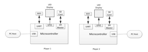
A block diagram of the system is shown above. The LED display is driven by the GPIO pins of the microcontroller and the WiFi module is connected to a UART in the microcontroller. The SD card is interfaced to the microcontroller through a SPI master block. User input is from the keyboard on the host PC.
