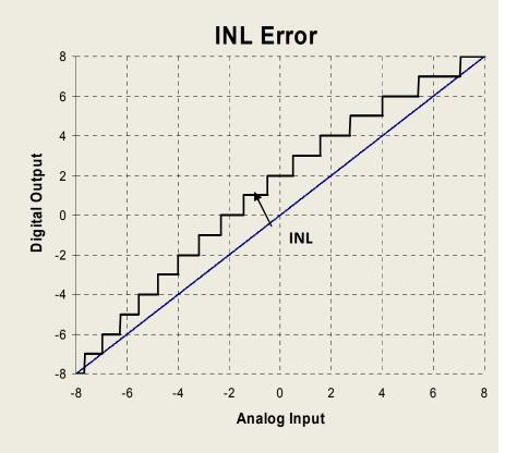
INL is a function of each ADC's particular architecture. It is not possible to remove its effects with calibration.
