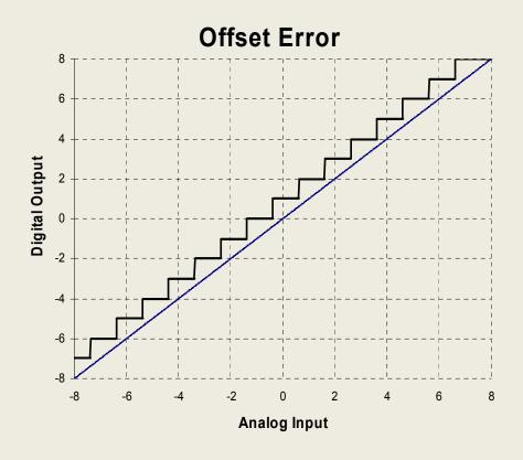
Offset error can be removed be measuring a reference point and subtracting that value from future samples.
