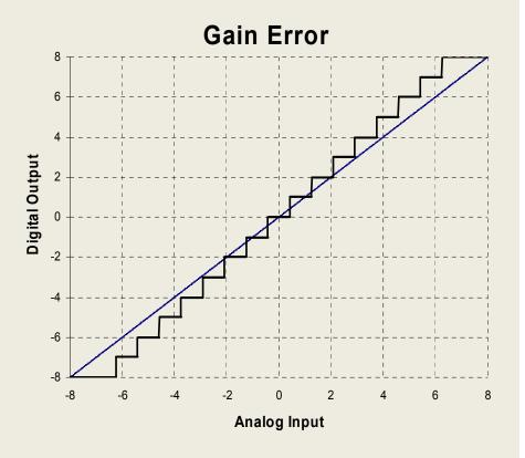
Gain error can be removed be measuring a second reference point to determine the actual gain.
