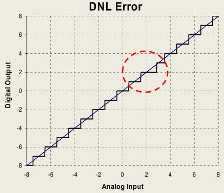
DNL is a function of each ADC's particular architecture. It is not possible to remove its effects with calibration.
