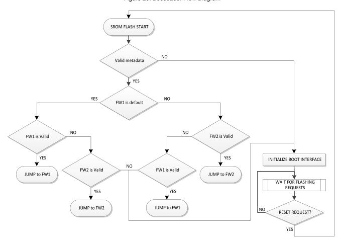
Since CCGx uses redundant firmware images that can update each other, it is expected that the device always has at least one functional image that can be booted by the bootloader. The programming through bootloader capability in notebook and dongle applications will only be used when using a CCGx part programmed with only the bootloader at factory.
