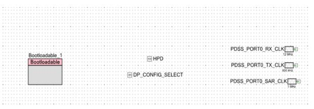
Open TopDesign.cysch file in the PSoC creator project to access dongle's schematic. Schematic contains hardware resources used by dongle such as clocks, Hot Plug Detect IO etc.
