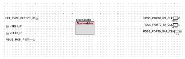
Open TopDesign.cysch file in the PSoC creator project to access power adapter's schematic. Schematic contains hardware resources used by power adapter such as clocks, voltage selection IOs etc.
