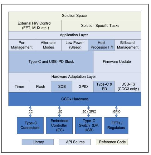
The CCGx firmware architecture contains the following components:
