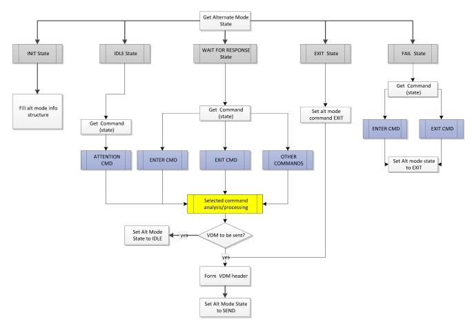
Figure 31: Alternate mode handler state machine for DFP
