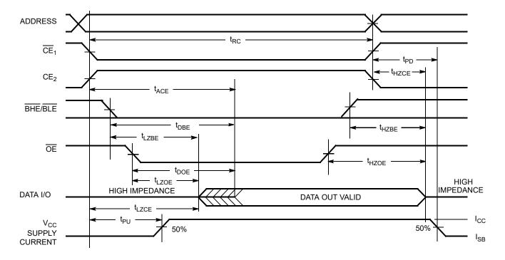
Notes 26. The device is continuously selected.  $\overline{OE}$ ,  $\overline{CE}_1 = V_{IL}$ ,  $\overline{BHE}$ ,  $\overline{BLE}$  or both =  $V_{IL}$ , and  $CE_2 = V_{IH}$ .
