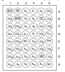
Figure 2. 48-pin TSOP I Pinout (Top View)[2, 3]
