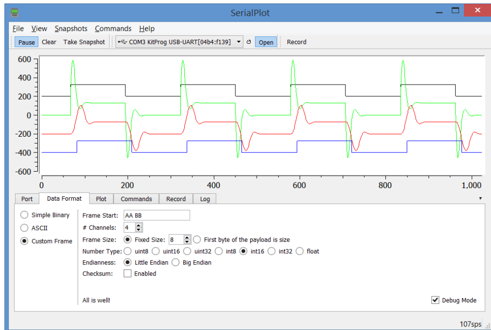
Figure 8. Filter response to the square wave with transition artifacts. Filter length is 31. Black line – signal w/o noise; Green – signal with noise; Red – FIR output; Blue – median filter output (recovered data). Vertical offsets are added for clarity. Data Format panel displays configuration settings.
