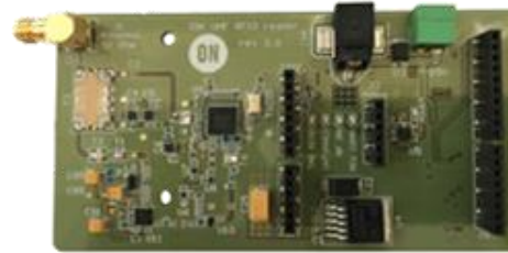
Smart Passive Sensor Reader Board SPS-Reader-GEVK
