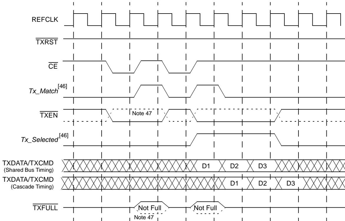
**Figure 9. Transmit Selection with Transmit FIFO Bypassed**
