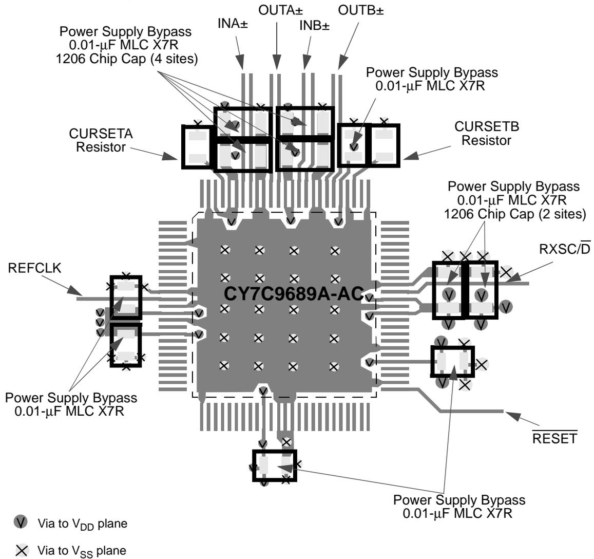
This is a typical printed circuit board layout showing example placement of power supply bypass components and other components mounted on the same side as the CY7C9689A.
