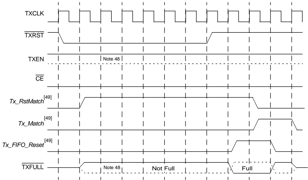
**Figure 13. Transmit FIFO Reset Sequence with Constant  $\overline{CE}$**
