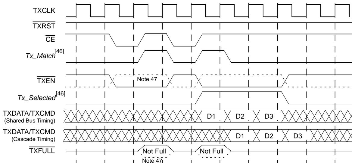
**Figure 8. Transmit Selection with Transmit FIFO Enabled**
