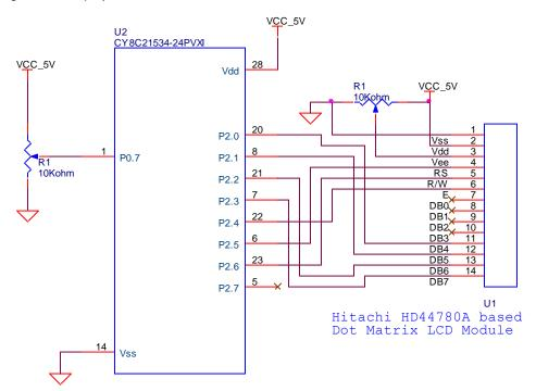
The LCD is connected to Port2 of the PSoC<sup>®</sup> chip CY8C21X34. The analog input is connected to P0[7]. The project can be tested by varying external 0 to 4 V between  $V_{SS}$  and P0.7.
