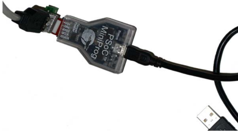
Figure 2. Components Use for Re-programming an enCoRe II Based Device
