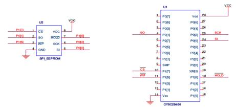
The code example uses CY8C29466 PSoC1 microcontroller. This code example can be tested using the CY3210 Eval board.
