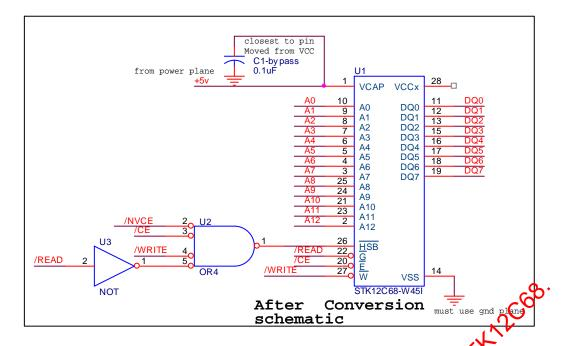
On the next page, pin by pin comparisons of the two show all pins are the same except for the two additional address lines.
