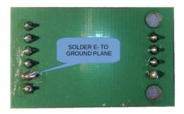
Figure 14. Options for repair HX711 PCB board: left – the E- terminal connected to GNP pin using wire; right – the E- terminal connected directly to the ground plane with a solder blob.
