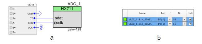
Figure 5. Pins configuration: (a)- component appearance on schematic, (b)- pins assignment. The off-chip annotation component is provided merely for illustration purpose; its presence on the schematic does not affect operation of the component.
