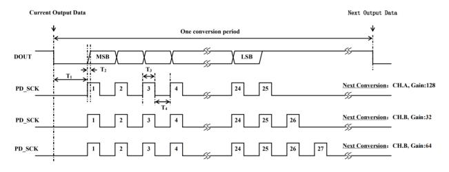
Figure 3. Data reading and gain selection timing [1].
