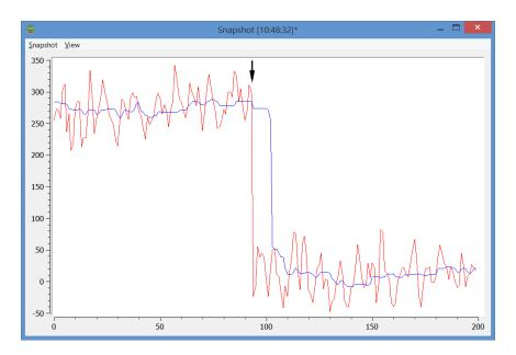
Figure 11. Load scale tare (zero) using a switch button. Button press event is marked by the arrow.
