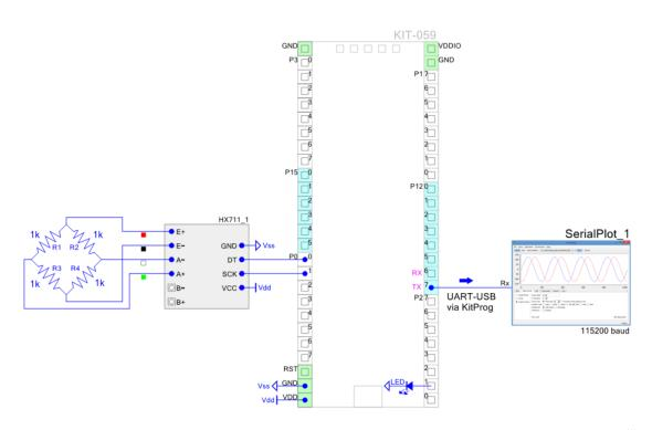
Figure 13. Schematic example for HX711 and CY8CKIT-059 using PSoC Annotation library<sup>(\*)</sup>.
