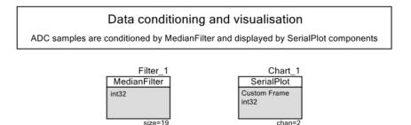
Figure 8. Data conditioning and plotting using MedianFilter and SerialPlot components.
