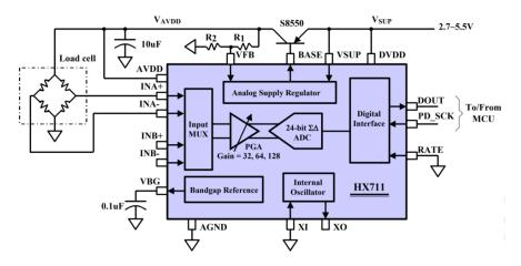
Figure 2. HX711 standard wiring diagram. The LPFs and rate selection resistor are not shown.
