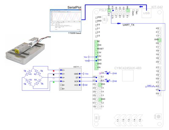
Figure 7. HX711 ADC board connection to the PSoC4 Pioneer Board (CY8CKIT-042) using KIT-042 annotation stub<sup>(\*)</sup>.
