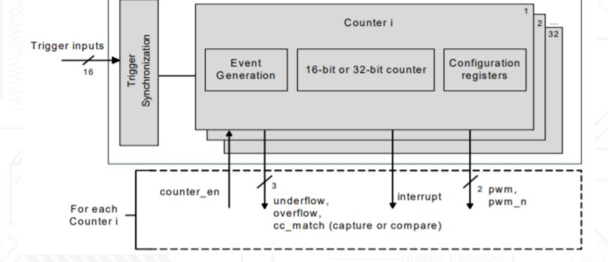
Interrupts: Provides interrupt request signals from each counter, based on TC or CC conditions
